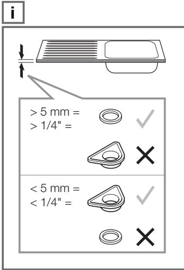
The diagram shows a sink with a callout box containing a table of gasket selection criteria. The table lists four options based on gasket thickness and shape, with checkmarks for correct and crosses for incorrect choices.
