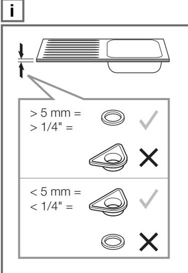
The diagram shows a sink with a callout box containing a table of gasket selection criteria. The table lists four options based on thickness and diameter, with checkmarks for correct and crosses for incorrect choices.
