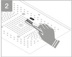
Only apply the cleaning agent to the toothbrush, never to the product, as the spray mist can penetrate openings and crevices and cause damage.
