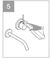
It is important to rinse thoroughly with clean water after each cleaning until all residues of the cleaner have been removed and then dry the product.
