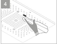
It is important to rinse thoroughly with clean water after each cleaning until all residues of the cleaner have been removed and then dry the product. The same applies to the COOL-MIST spray nozzle and the laminar spray.
