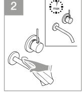
Only apply the cleaning agent to the cleaning cloth, never to the product, as the spray mist can penetrate openings and gaps and cause damage.
